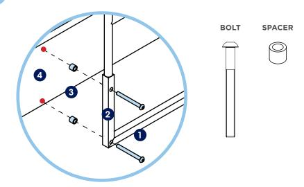
Tighten each bolt (x4 total) with a 5mm Allen Key or using an electric drill (with 5mm hex bit), to secure.
